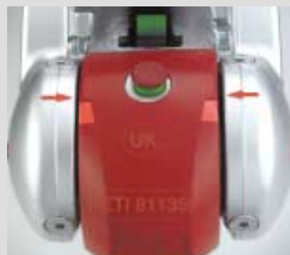
Friction Pads are worn out & need replacing
