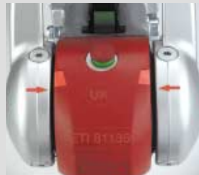
Friction Pads are in good order
